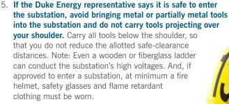
Don't climb. Always maintain the necessary clearance from the overhead conductors. After the Duke Energy representative deems it safe to enter, stay on the ground for your own safety.
